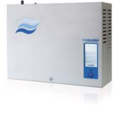
Condair RM Low capacity resistive humidifier Offers 2-8kg/h of steam for in-duct humidification.
